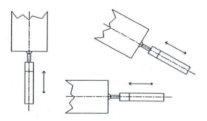
3. Torsional forces or forces which can affect the device at a slanted angle can lead to damages of the measuring tool.
